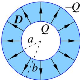
A spherical capacitor consists of two conducting spheres of radii  $a$  and  $b$  ( $a < b$ ) with dielectric of constant  $\kappa$  in between (diagram shows the cross section).
