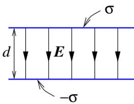
A parallel plate capacitor consists of two parallel planar conductors separated by distance  $d$ . The electric field in this system is found as a superposition of the fields of two uniformly charged planes (Example 2 in Sec. 1.7) with surface charge densities  $\sigma$  and  $-\sigma$ . The fields outside the plates cancel, and the fields between them add to give
