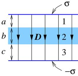
Consider a parallel plate capacitor in which a layer of dielectric of thickness  $b$  and dielectric constant  $\kappa$  is inserted parallel to the plates and separated from them by vacuum gaps of thickness  $a$  and  $c$  (see diagram).
