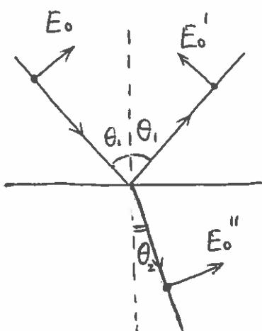
Let the wave be now polarised in the direction parallel to the plane of incidence. Choosing the amplitudes of the magnetic field,  $H_0$ ,  $H_0'$  and  $H_0''$  towards us (perpendicular to the page plane), we have the electric field amplitudes as shown on the diagram.
