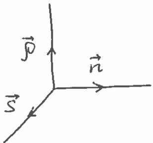
( $\vec{p}, \vec{s}, \vec{n}$ ) is the right-handed set of vectors (rotation from  $\vec{p}$  to  $\vec{s}$  is anticlockwise, if viewed from top of  $\vec{n}$ ). (6)
